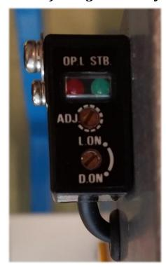
To adjust the sensitivity of the sensor turn the dial marked ADJ on the sensor with a small screwdriver. Test the sensitivity in both up and down mode until you find a settings that works well for both.
