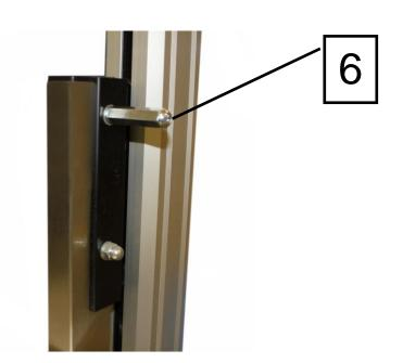
Remove the nut from the top bolt holding the attachment to the slide and replace it with the extra-long nut (6). Use the manual control to raise the attachment and make sure the extra-long nut trips the breaker arm (3) before the slide reaches the top of the mast. The lifter should stop when the breaker arm is triggered and only lowering will be allowed.
