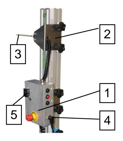
First slide the box (1) into the slot on the back of the mast and tighten the black nob to hold it in place, and then slide the top breaker (2) into the same slot. The breaker arm (3) must be at least 120mm from the top of the mast. Plug the hand control that came with the lifter into the 5-pin connector on the box (4). Plug the 5-pin connector from the box into the power pack on the lifter
