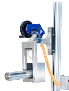
Expand&Turn - pneumatic expander, turning operated manually
