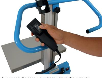
from very slow to medium before it reaches its full speed. Release your finger from the potentiometer and the load will smoothly stop.
